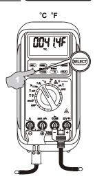
Note: insert the banana plug K-type temperature bead probe (stadard accessory x 1) with correct + - polarities. Dual channels T1-T2 readings require 2 probes. You can also use a plug adapter (Optional purchase) with banana pins to K-type socket to adapt other standard K type mini plug temperature probes.
